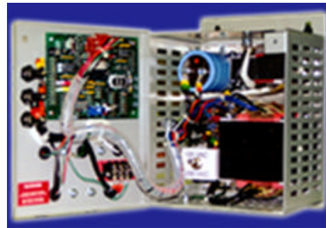
Modular component plate with point to point wiring.
